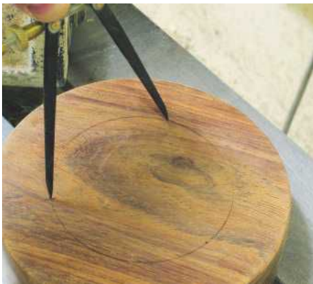
▲ Pic.10 The marked circle on the top surface is the centre of the three holes. Les could have used the lathe indexing but dividers made a simple job of finding the hole positions
